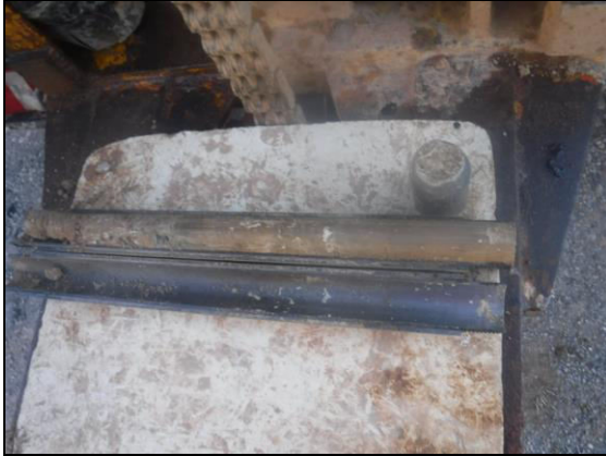
Foto 25: Sondeig S-10, SPT a 1,0 metre.
