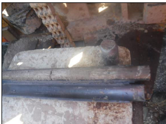
Foto 17: Sondeig S-7, SPT a 1,0 metre.
