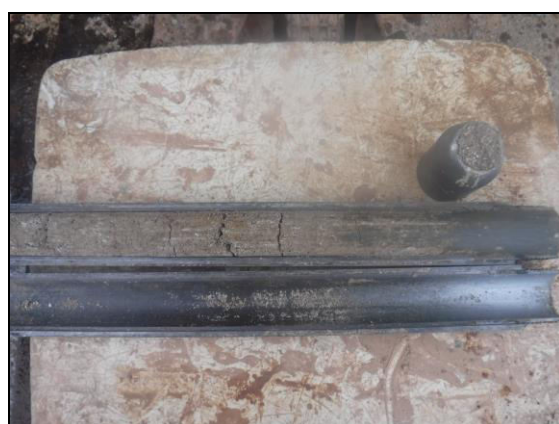
Foto 12: Sondeig S-5, SPT a 1,0 metre.
